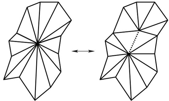
FIGURE 7. Expansion (respectively contraction) of an edge.
