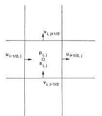
Fig. 3. The computational grid
