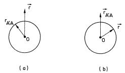
**Fig. 4a and b.** Source spheres: **a** The extremity of  $\mathbf{r}_{A'A}$  describes the whole sphere of radius  $r_{A'A}$  when curve  $\gamma$  rotates. The Newtonian field is created at **r** and vanishes inside the sphere. **b** The complementary situation: the extremity of **r** describes a sphere of radius *r* and the Newtonian field is created at  $\mathbf{r}_{A'A}$
