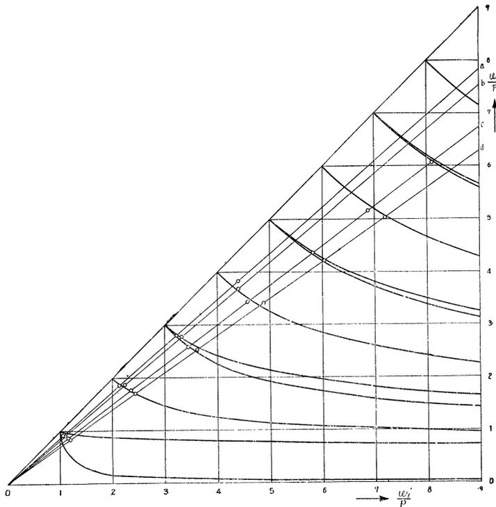
Fig. 3. Instability points in experiments are present nearly in instability ranges known from theory.
