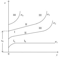
FIGURE 1: Various types of creep curves.
