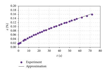
FIGURE 4: Creep curve of asphalt concrete at stress  $\sigma_0 = 0.19$  MPa.
