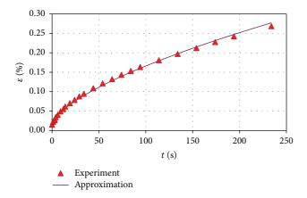
FIGURE 3: Creep curve of asphalt concrete at stress  $\sigma_0 = 0.16$  MPa.
