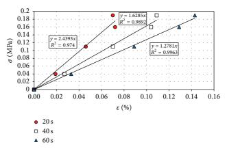
FIGURE 2: Isochronous lines of deformation of asphalt concrete.
