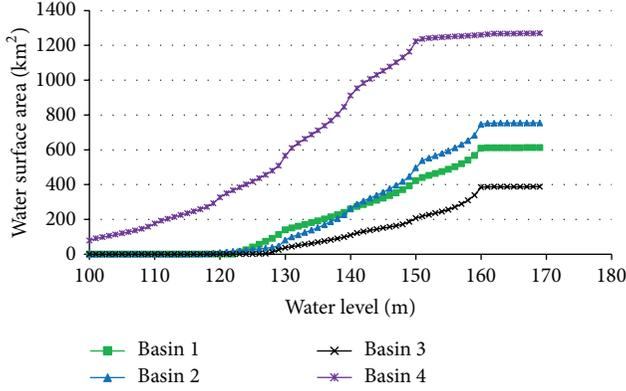
FIGURE 4: Topographic relation of water surface area versus water level.
