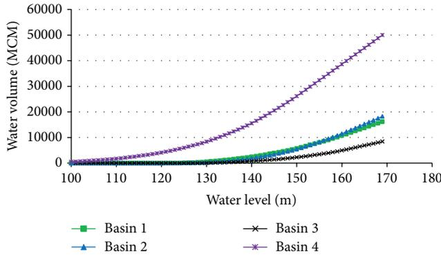
FIGURE 5: Topographic relation of water volume versus water level.
