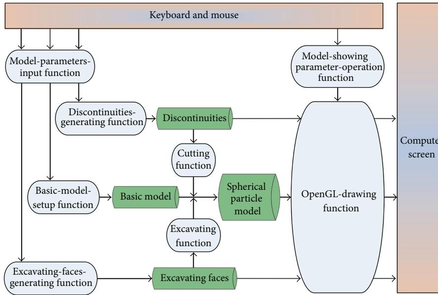
FIGURE 1: Program structure of the SGIM.
