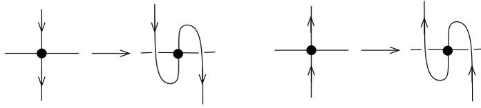
Fig. 16. Local changes at a vertex of the core graph to remove a half-twist. On the left, the path  $P$  originally traverses the vertex top-to-bottom. It is made to traverse the vertex bottom-to-top instead, altering  $P$  only in a neighborhood of the vertex. Likewise, on the right, a bottom-to-top traverse is switched to a top-to-bottom traverse by altering  $P$  locally.
