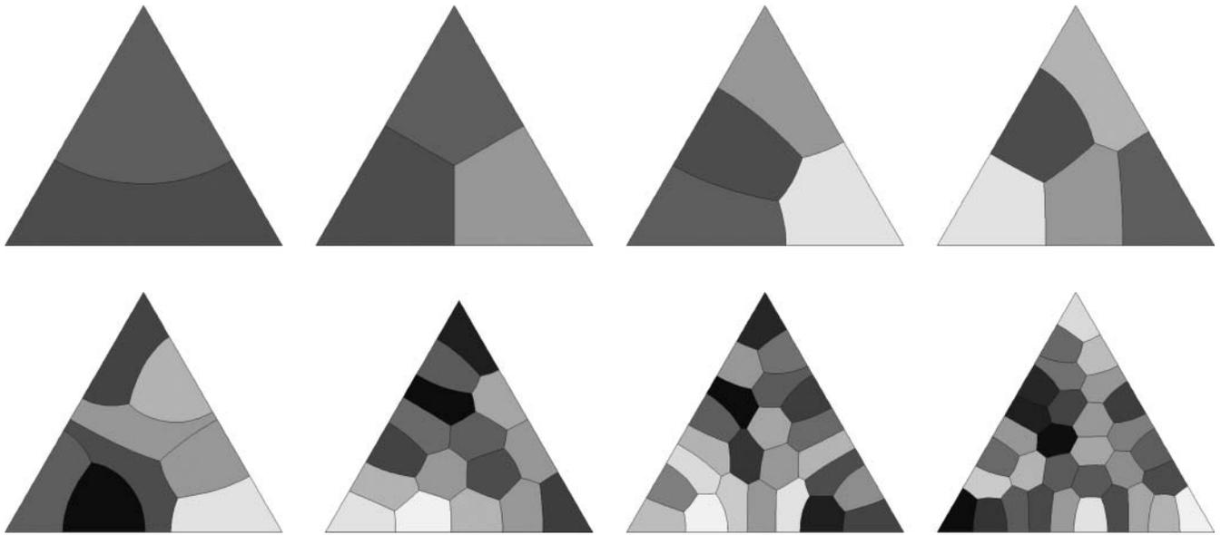
FIGURE 3. Tiling of the triangle with 2, 3, 4, 5, 8, 16, 24, 32 cells.
