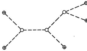
Fig. 3. A typical link with hinges  $(\oplus)$ , knots  $(\circ)$ , and chains (----)
