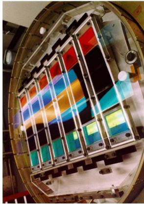
FIG. 7. The SDSS camera. Its CCDs—each  $2048 \times 2048$  pixels—are arranged in six columns and five rows. A different filter covers each row. Credit: SDSS (2018b).
