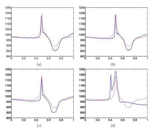
FIG. 2. Patient Sel104—case of cardiac arrhythmia. Solid and blue curves: four signals containing a single QRS complex out of J=285 extracted from the ECG recording displayed in Figure 1. The length of the signals is n=128 time points. Dashed and red curve: Euclidean mean of the raw data. Units on the horizontal axis are arbitrary.
