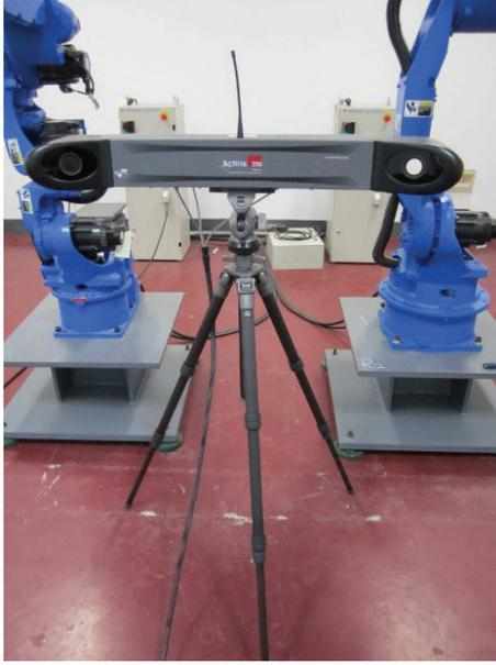
FIGURE 10: 3D coordinate measuring machine Actiris350.
