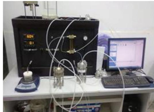
FIGURE 6: Servo flow permeameter.
