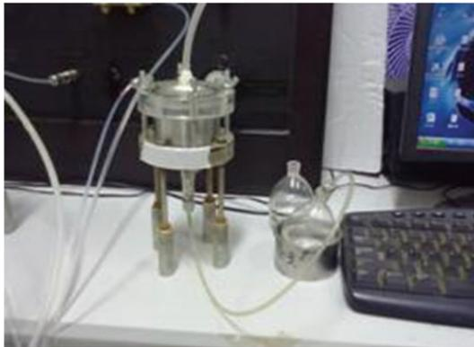
FIGURE 5: Outlet and evaporation correction bottle.
