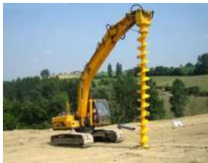
Contemporary auger is the same Archimedean screw still used after more than 2000 years
