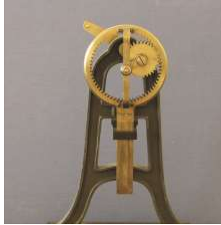
Planetary gear or Tusi couple mechanism (Kinematic model collection, Cornell University, photo Prof. Francis Moon)
