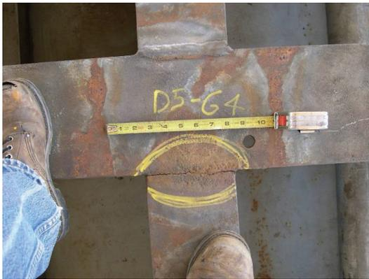
FIGURE 6: Fatigue crack in diaphragm flanges of miter gate.
