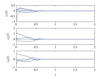
FIGURE 1: Evolution process of synchronization errors of two Chua's circuit networks.
