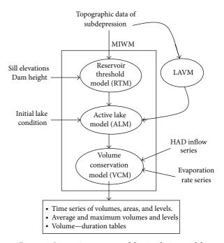
FIGURE 3: Interactive structure of the simulation model.
