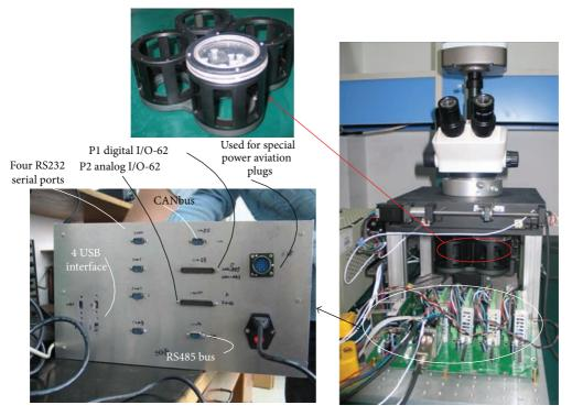
FIGURE 14: A photograph of cell culture and observation system platform.
