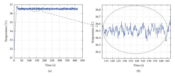
FIGURE 18: (a) Temperature characteristic of temperature closed-loop control circuit with start temperature at 31.65°C. (b) Temperature characteristic partial enlarged detail.
