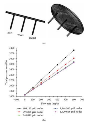
FIGURE 8: The grids method: (a) the side view of mesh division for cell culture internal cavity, (b) the curve result of the flow rate for outlet total pressure loss.
