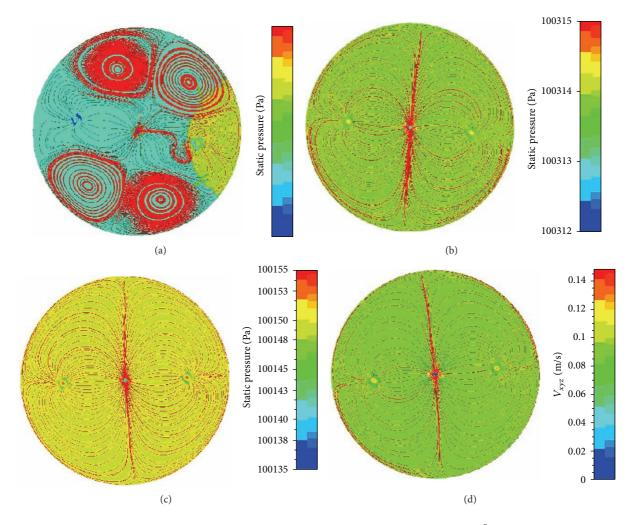
FIGURE 12: The simulation results of micro flow: (a) the flow field distribution when the flow rate is  $3 \times 10^{-7}$  kg/s, (b) the flow field distribution when the flow rate is  $3 \times 10^{-5}$  kg/s, (c) the flow field distribution when the flow rate is  $3 \times 10^{-4}$  kg/s, (d) the flow field distribution when the flow rate is  $2 \times 10^{-7}$  kg/s.
