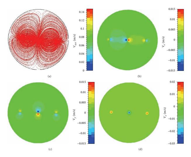
FIGURE 11: The simulation analysis when the flow rate is 200 mg/s. (a) Streamline distribution, (b) velocity distribution in *x* direction, (c) velocity distribution in *y* direction, (d) velocity distribution in *z* direction.
