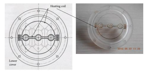
FIGURE 6: The engineering drawing for lower cover of cell culture cavity.
