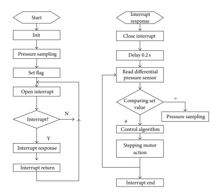
FIGURE 16: Micro fluid controlling software flow chart.
