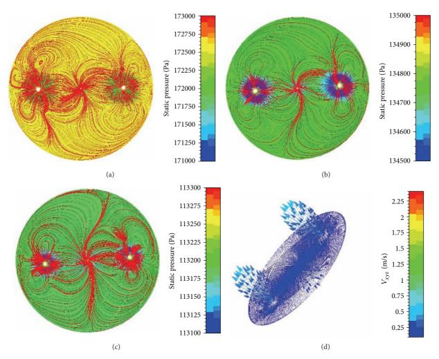
FIGURE 9: The simulation results in large flow: (a) the middle surface streamline chart in inlet static pressure of 200,000 Pa, (b) the middle surface streamline chart in inlet static pressure of 150,000 Pa, (c) the middle surface streamline chart in inlet static pressure of 120,000 Pa, (d) the middle surface vector of cavity in inlet static pressure of 150,000 Pa.
