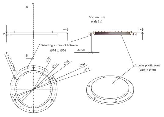
FIGURE 5: The engineering drawing for upper cover of cell culture cavity.
