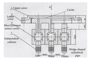
FIGURE 4: The assembly drawing of cell culture cavity.
