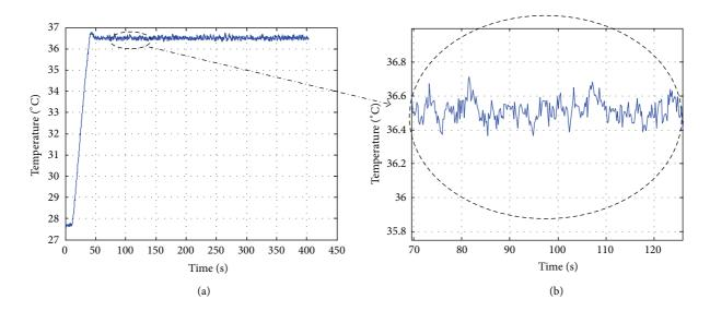
FIGURE 17: (a) Temperature characteristic of temperature closed-loop control circuit with start temperature at 27.68°C. (b) Temperature characteristic partial enlarged detail.
