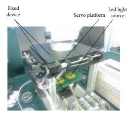
FIGURE 7: A photograph of cell culture cavity three-dimensional servo platform.
