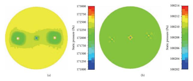
FIGURE 10: The pressure distribution graph of cell culture cavity: (a) the middle surface pressure distribution graph in inlet static pressure of 200,000 Pa, (b) the pressure field distribution when the flow rate is  $2 \times 10^{-4}$  kg/s.
