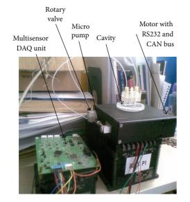
FIGURE 15: A photograph of micro pump and multisensor data acquisition unit.
