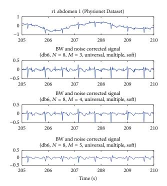
FIGURE 9: r1 abdomen 1 Abdominal and Direct Fetal Electrocardiogram Database (Physionet Dataset) signal and BW and noise corrected signals using different levels for denoising.
