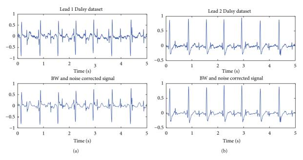
FIGURE 6: Dalsy database signals: (a) lead 1 and noise and BW corrected signal; (b) lead 2 and noise and BW corrected signals.
