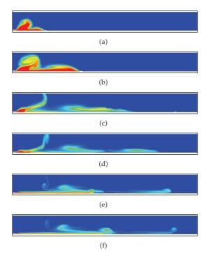
**Figure 8:** Series numerical images of species distributions near muzzle region by the gunshot of unsuppressed rifle in Case 1: (a) 0.82 ms, (b) 1.0 ms, (c) 1.5 ms, (d) 2.0 ms, (e) 2.5 ms, and (f) 3.0 ms.
