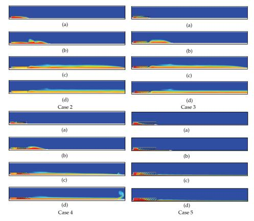
**Figure 9:** Series numerical images of species distributions near muzzle region by the gunshot of suppressed rifle in Case 2–Case 5: (a) 0.82 ms (b) 1.00 ms (c) 2.00 ms (d) 3.00 ms.
