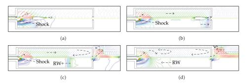
Figure 11: Distributions of pressure and velocity vectors in Case 2 (a)  $0.72 \, \text{ms}$ , (b)  $0.80 \, \text{ms}$ , (c)  $0.86 \, \text{ms}$ , and (d)  $0.90 \, \text{ms}$ .
