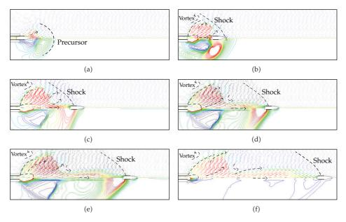
Figure 10: Distributions of pressure and velocity vectors in Case 1 (a)  $0.68\,\mathrm{ms}$  (b)  $0.72\,\mathrm{ms}$  (c)  $0.76\,\mathrm{ms}$  (d)  $0.80\,\mathrm{ms}$  (e)  $0.84\,\mathrm{ms}$  (f)  $0.88\,\mathrm{ms}$ .
