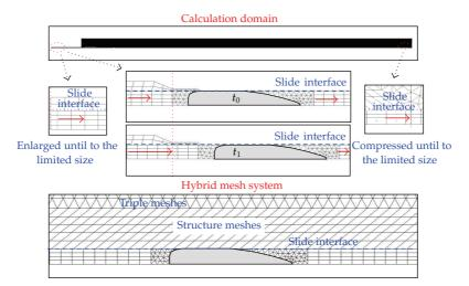
Figure 3: Description of generation of moving grids.
