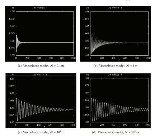
Figure 2: Stretch ratio with varying *N*.
