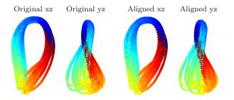
FIG 4. Registration of juggling cycles for one of the trials in the dataset. We provide two different views for improved display. The cumulative variance decreased from 9.05 to 3.77 due to cycle registration.
