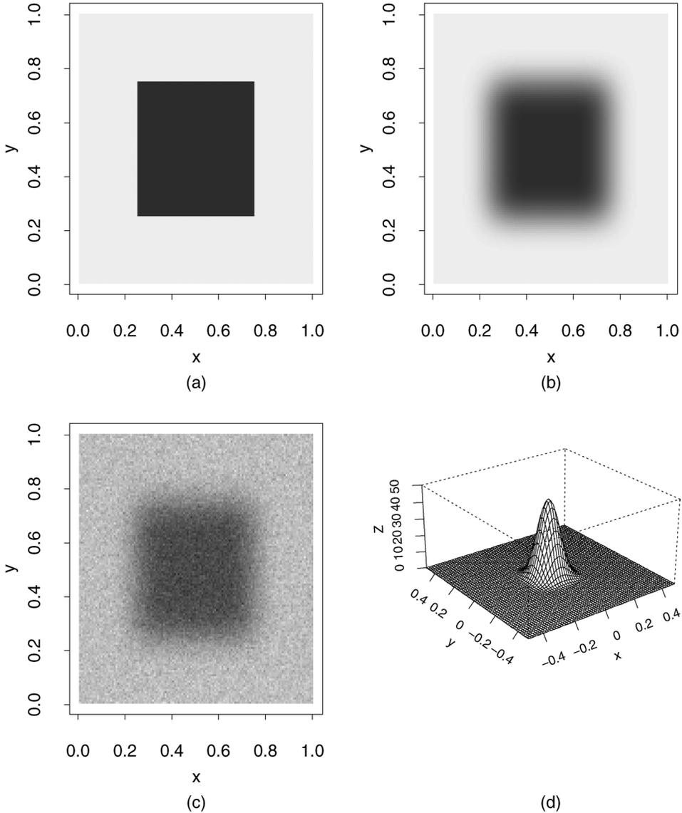
FIG. 1. Graphs of  $\psi$ ,  $\phi$ ,  $\phi\psi$  and  $Y$ . Panel (a) shows the true image,  $\psi$ . Panel (b) shows its blurred version,  $\phi\psi$ . The function  $\phi$  itself is depicted in panel (d). Panel (c) shows the blurred image plus noise; the latter was  $N(0, 0.1^2)$  on each pixel. Digitization was on a  $128 \times 128$  grid.
