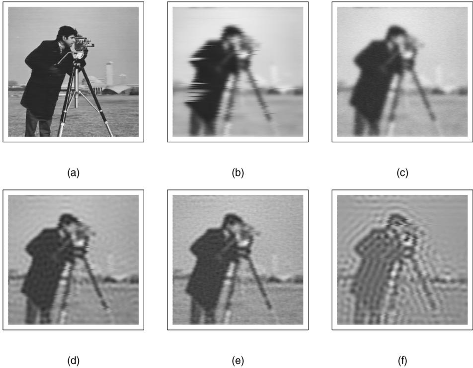
FIG. 3. *Cameraman example.* Panels (a)–(c) show the original, the blurred, and the blurred-and-noisy cameraman images, respectively. Panels (d) and (e) show images restored from (c) by the inverse filter and the Wiener filter, respectively. Panel (f) shows the restored image, obtained by the Wiener filter, when a Gaussian point-spread function with standard deviation  $\lambda/2$  was used in deblurring.
