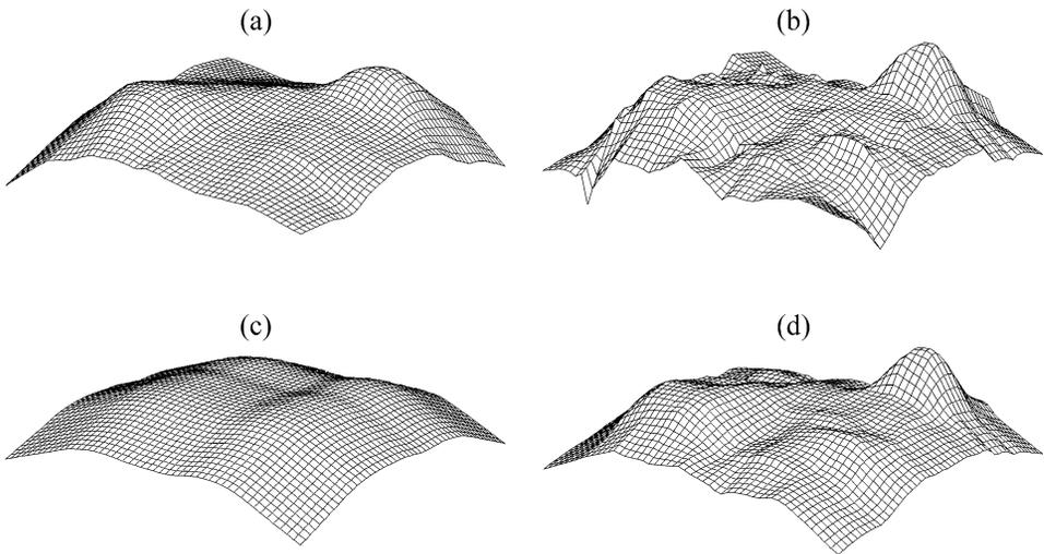
FIG. 2. Comparison of different estimators. The local linear estimator is either heavily biased (a) ( $h = 0.174$ ,  $R = 0$ , ISE = 8.3) or wiggly (b) ( $h = 0.117$ ,  $R = 0$ , ISE = 8.8). Additive estimation (c) ( $h = 0.197$ ,  $R = \infty$ , ISE = 17) is even worse. The penalized estimator (d) ( $h = 0.117$ ,  $R = 0.163$ , ISE = 6.0) is stabilized without oversmoothing: ISE is improved by more than a quarter.
