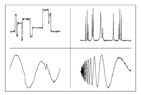
FIG. 4. SURESHRINK reconstruction using S8 wavelets.
