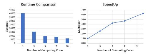
FIG. 5. Runtime comparison in seconds and speed up with varying number of computing cores.
