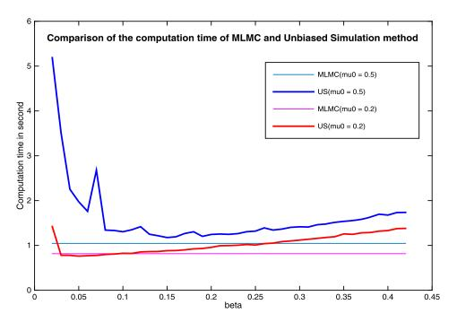
FIG. 1. Comparison of the computation time of MLMC method and unbiased simulation method for problem (4.3), with the same given error.
