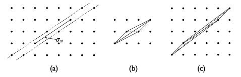
FIG. 6. Flips of an edge  $\sigma_x$ . (a) Possible locations of the third vertex of the triangles containing  $\sigma_x$  are the integer points on the dotted lines. (b) Unique flip of  $\sigma_x$  to a shorter edge ( $\sigma_x$  is the diagonal of its minimal parallelogram). (c) A flip of  $\sigma_x$  to a longer edge.
