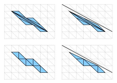
FIG. 10. The region  $\Upsilon(\sigma_x)$  when  $\sigma_x$  is an edge of slope (-3, 5) (with midpoint in the center of the box). Left: in the case of no constraints. Right: in the presence of a constraint edge of slope (-4, 7). Above: the triangles inside correspond to the second definition of the influence region. Below: the triangles inside correspond to the first definition of the influence region. In the background, a ground state triangulation (dotted lines).
