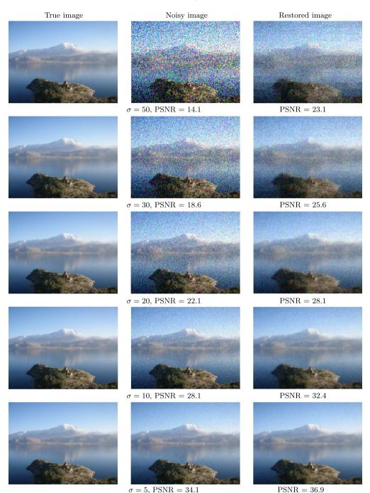
Fig. 2. The result of the experiment on image densoising. Left: the original  $120 \times 160 \times 3$  image. Middle: the noisy image for different values of  $\sigma$ . Right: the denoised image.
