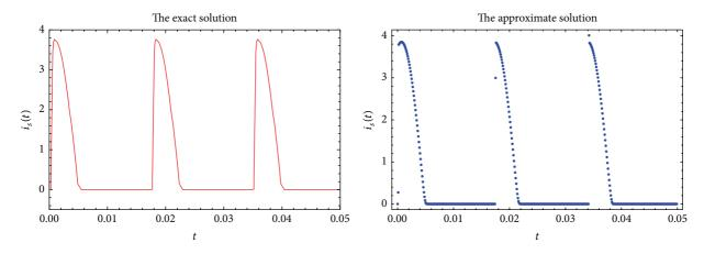
FIGURE 2: The exact and approximate solutions for the current of the diode circuit.
