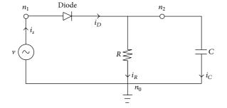
FIGURE 1: Rectifier circuit.
