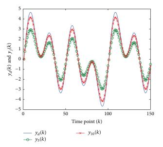
FIGURE 7: Example 2, the reference  $y_d(k)$  and output  $y_j(k)$  for j = 5 and j = 10.
