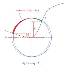
FIGURE 9: Deriving  $\partial g/\partial s$  as the difference in heights of the entry and exit points.
