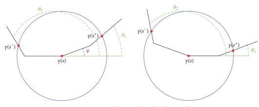
FIGURE 11: Using  $g_{s-}$  and  $g_{s+}$  to obtain the polygon angle at *s*.
