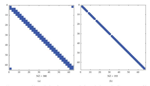
FIGURE 1: (a): Sparsity pattern of the periodized transform matrix  $T_{\text{Daube}}$  by the periodized D4 wavelets; (b): sparsity pattern of the inverse transform matrix  $T_{\text{cubic}}^{-1}$  of the cubic spline wavelet.
