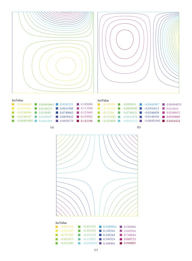
FIGURE 3: Contour plots of numerical solution by one-level method. From (a) to (c): two components of velocity and pressure.
