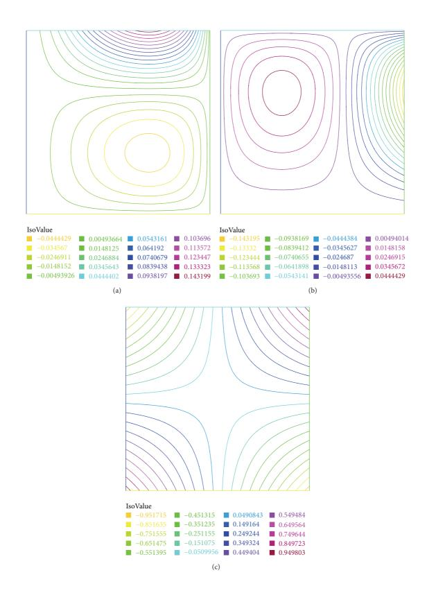
FIGURE 4: Contour plots of numerical solution by two-level Newton method. From (a) to (c): two components of velocity and pressure.
