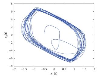
FIGURE 1: Chaotic behavior of master system (3) with u(t) = 0.
