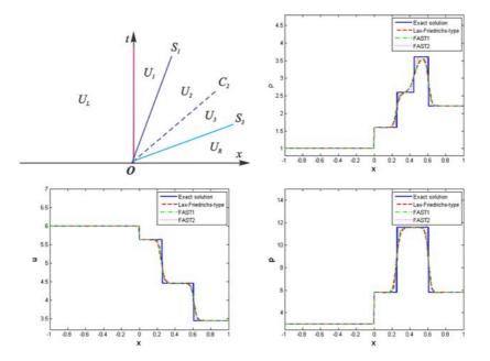
Fig. 4. Test 3: Approximate solution by the Lax-Friedrichs-type, FAST1, and FAST2 schemes with 500 mesh points on the interval [-1;1].
