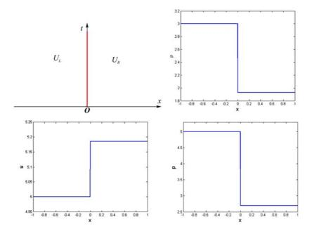
Fig. 1. Test 1: Approximation of a stationary contact wave by FAST2 scheme at the time t = 0.1 with 500 mesh points on the interval [-1; 1].
