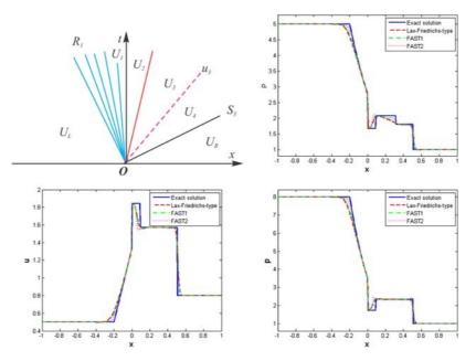
Fig. 6. Test 4: Approximate solution by the Lax-Friedrichs-type, FAST1, and FAST2 schemes with 500 mesh points on the interval [-1;1] at the time t = 0.2.
