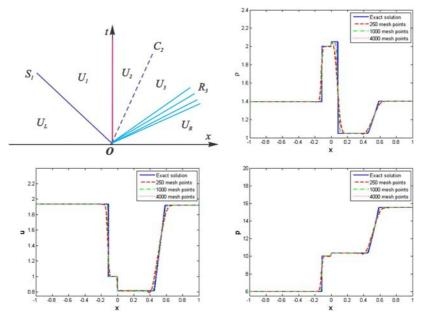
Fig. 3. Test 2: Approximate solution using the underlying FAST2 numerical ux. The approximate solution is computed at the time t = 0.1 on the interval [-1; 1] with 250, 1000, and 4000 mesh points, and is compared with the exact solution.
