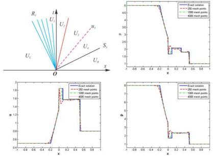
Fig. 7. Test 4: Approximate solution using the underlying FAST2 numerical ux. The approximate solution is computed at the time t = 0.2 on the interval [-1; 1] with 250, 1000, and 4000 mesh points, and is compared with the exact solution.
