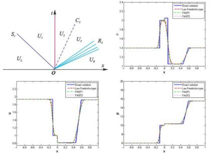
Fig. 2. Test 2: Approximate solution by the Lax-Friedrichs-type, FAST1, and FAST2 schemes with 500 mesh points on the interval [-1; 1].
