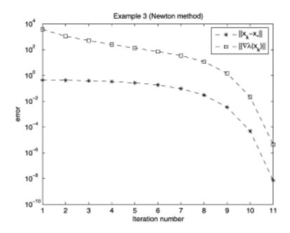
Fig. 11. Numerical results for Example 3 by Newton's method with initial guess  $[0.1 \ 0.4 \ 1.0]^T$ .
