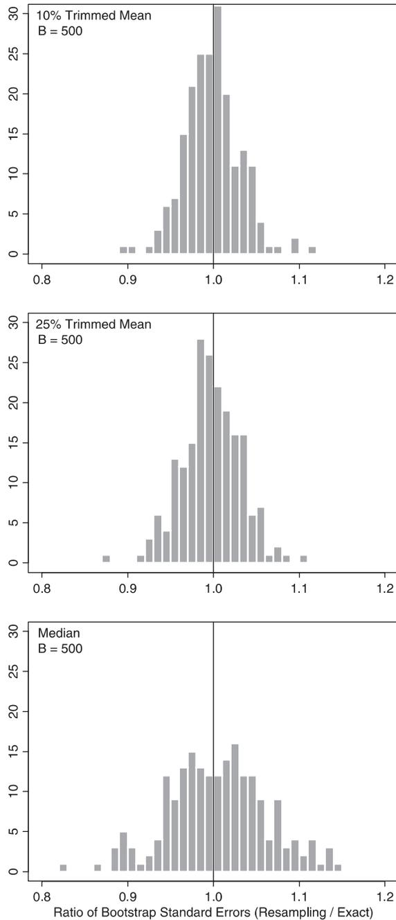
FIG. 2. Ratio of 200 bootstrap standard errors, based on  $B = 500$  resamples each, to the exact bootstrap standard error of the 10% trimmed mean, 25% trimmed mean and median of the data in Table 1.
