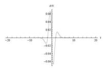
Figure 6: Wavelet  $\psi(t) = D^{(5)} \left[\frac{1}{2\pi}\operatorname{sech}(t/2)\right]$
