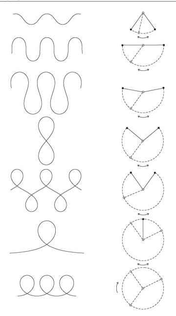
**Figure 1.** The elastic curves produced via formulas (22). In all cases the parameter  $\lambda$  is fixed, i.e.,  $\lambda = 4$ . The first five figures starting from the top on the left hand side are generated by (22 A) and following values of  $\mu$ : 0.5, 0, -0.4, -0.65223 and -0.9. The sixth one represents (22 B) while (22 C) in conjunction with  $\nu = 1.2$  produces the last one.
