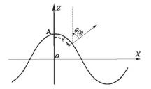
**Figure 4.** Geometry of the elastic curve in terms of the azimuthal angle  $\theta(s)$ .
