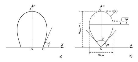
Figure 2. a) An elastic curve on the way to the figure "eight" shape. b) Geometry of the upper half of the figure "eight" elastica.
