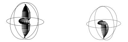
Fig. 2. Catenoid with  $p_0 = -q_\infty = 1$  and  $p_\infty = q_0 = 0$ , and  $\phi = \pi/2$ . The figure is the image of  $z = re^{i\theta}$  where  $e^{-3} < r < e^3$ ,  $0 \le \theta \le \pi$  and  $1 < r < e^3$ ,  $0 \le \theta \le \pi$ , respectively.
