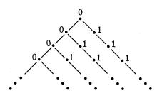
Any ips  $\{d_n\}$  of S is obtained by tracing a descending path in the tree. Define the integer valued function f on S as follows:
