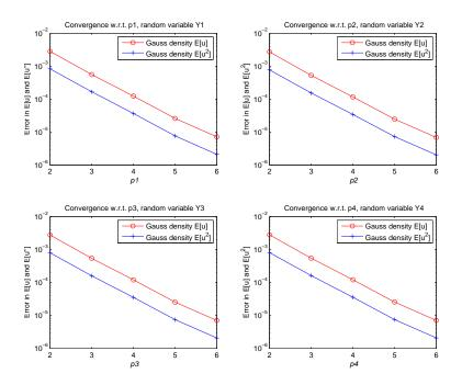
FIGURE 2. Convergence results for the approximation of expected value and second moment with Gauss density in Example 4.1.
