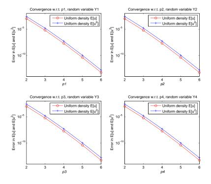
FIGURE 1. Convergence results for the approximation of expected value and second moment with uniform density in Example 4.1.
