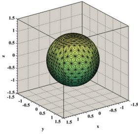
(a) Triangulation of a unit sphere with 512 faces.
