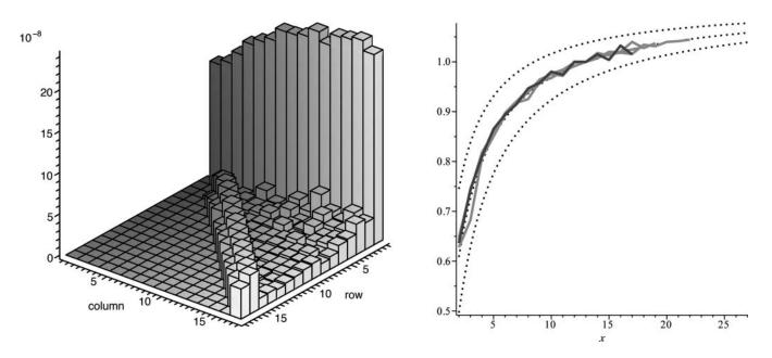
**FIGURE 2.** Left: Inverse computing times for our Monte Carlo method as a function of the block size. Right: Growth regimes associated with various block sizes. Dotted lines (from below) correspond to subexponential terms of order  $n^{-1}$ ,  $n^{-3/2}$ , and  $n^{-2}$ , respectively.
