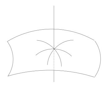
Unless the curvature of the curves through p is constant, one can prove that it takes a maximum value  $k_1$  and a minimal value  $k_2$  (called the principal curvatures) for perpendicular directions of the curves of intersection (called the principal directions at p).
