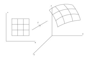
Technically, we suppose that  $f = (f_1, f_2, f_3)$  is smooth  $(C^{\infty})$ , that its differential is injective at each point and that it is a homeomorphism onto its image.
