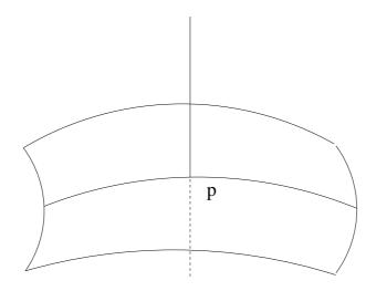
Now, rotate the plane around the normal. You get a family of curves and in general the curvature varies with the plane.
