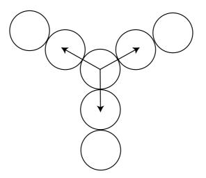
At first sight, no compact configuration would satisfy this condition but – remarkably – for a nodoid the  $\tau$  changes sign and the nodoid will "pull" and not "push". This can be loosely explained as follows. The push occurs at the junction of two spheres, and according to the configuration of unduloid or nodoid, it applies in opposite directions.
