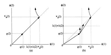
FIG. 3. The most likely scenario for the overflow of location 2 of the W network under the LLR policy, for the cases (a) q(1) = q(2), (b) q(1) > q(2).
