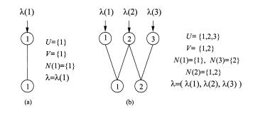
FIG. 1. Two load sharing networks of interest: (a) The single-location network, and (b) the W network.
