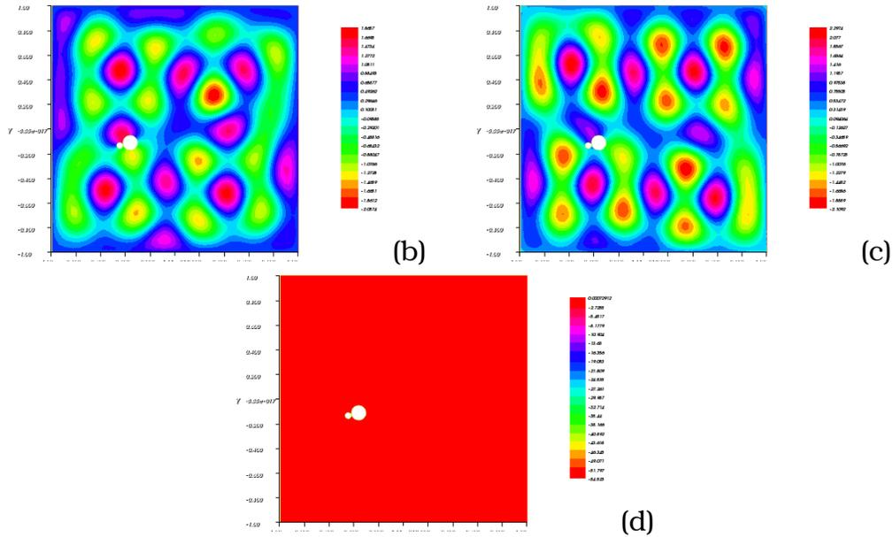
FIGURE 10. SECOND STEP : b) DIRECT STATE, c) ADJOINT STATE d) TOPOLOGICAL DERIVATIVE . Second step : b) Direct State, c) Adjoint state d) Topological derivative
