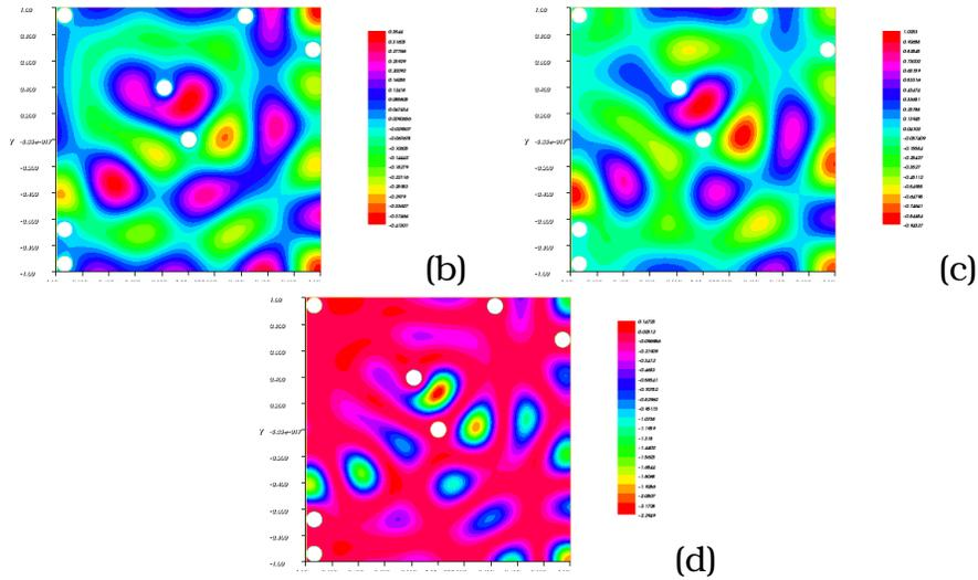
FIGURE 21. FIRST STEP: b)DIRECT STATE, c)ADJOINT STATE d)TOPOLOGICAL DERIVATIVE. First step: b)Direct State, c)Adjoint state d)Topological derivative
