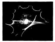
Caustics formed in the far field by a broadened laser beam incident on a water drop 'lens'.
